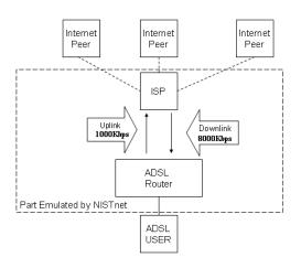
Figure 1. A P2P host running behind a bandwidth-asymmetric network
