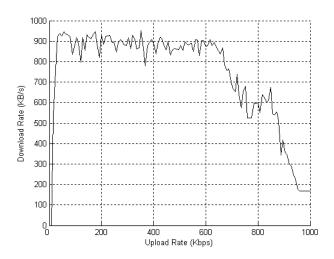
Figure 2. Effect of upload data rate on download throughput
