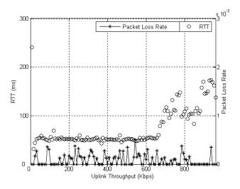
Figure 3. RTT and packet loss rate vs uplink throughput
