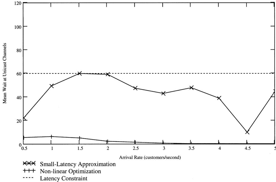
Fig. 6. Deviation of the small-latency approximation model under latency constraint of 60 s.
