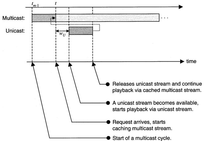
Fig. 3. Admission procedure for an admit-via-unicast client.
