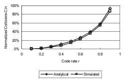
Fig. 10. Analytical and trace-driven simulated worst-case collisions against the code rate r.
