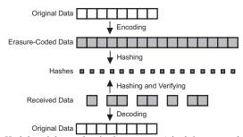
Fig. 2. Hash-based data authentication process. A hash is computed for each erasure-coded data block. The hashes are then distributed through a trusted channel.
