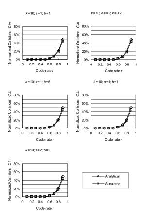
Fig. 8. Analytical and simulated average collisions against the code rate r.for number of peers k=10 with respect to different shape parameters a and b.
