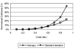
Fig. 11. Trace-driven simulated average collisions against the code rate r.
