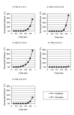
Fig. 9. Analytical and simulated average collisions against the code rate r.for number of peers k=100 with respect to different shape parameters a and b.
